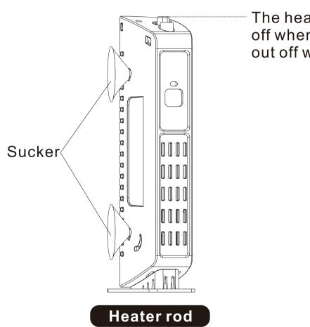
The heater will power off when this board is out off water
